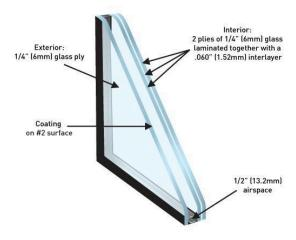
Figure 2 – Acoustic Glass Assembly
